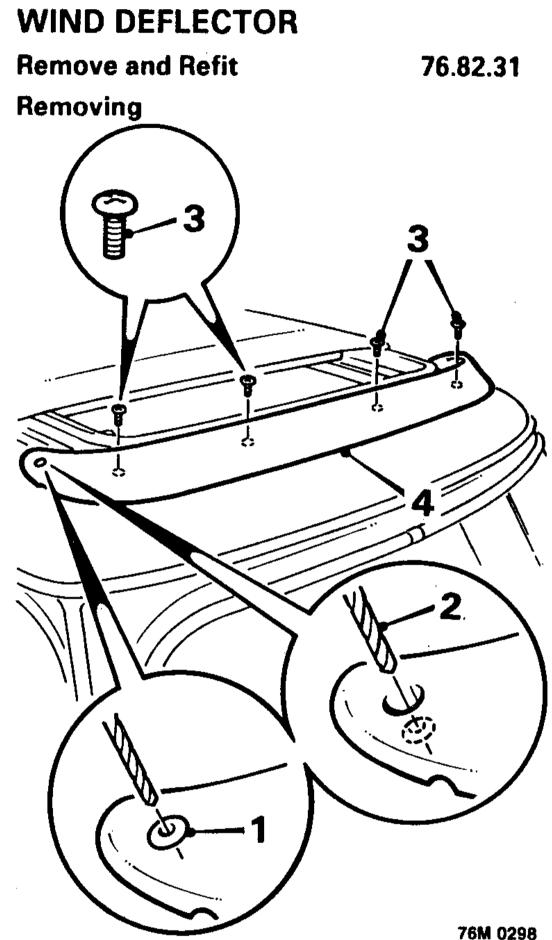
1. Remove 2 cover plugs by drilling a 3 mm hole through them and levering out with a small screwdriver.
