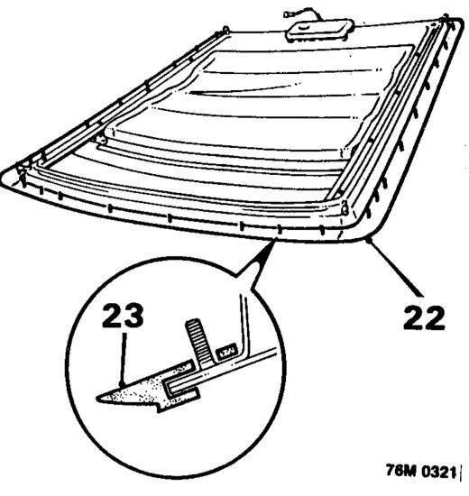
22. Remove sun roof assembly from vehicle.
