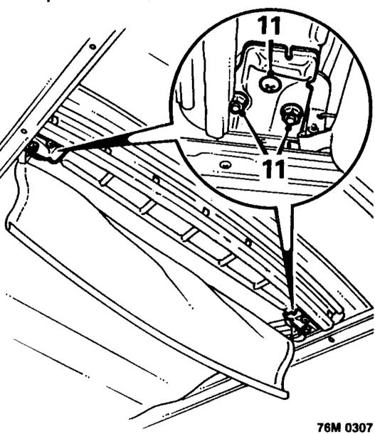
11. Remove 2 screws and 4 nuts securing cover assembly to drive cable blocks.
