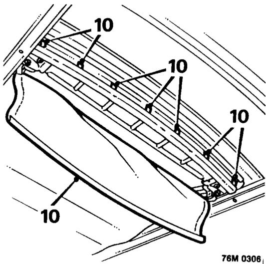
10. Push front of sun roof inner cover upwards to release from securing clips on frame.
