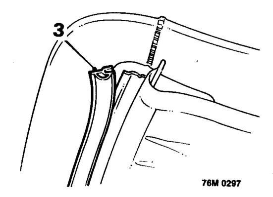
Carefully remove sun roof front seal from the outer cover support frame.
