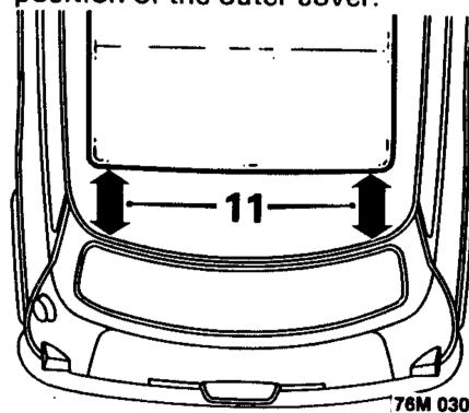
11. Measure between the rear edge of the outer cover and the roof drain channel to ensure both sides of the cover have been adjusted equally.
